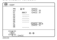
3 Press the ▼/▲ buttons to choose "CC" or "CH" according to the CH/ CC number of the TV channel
